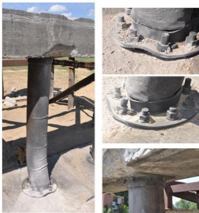
Figure 10: Global (Left) and Local Deformation (Right) of MSJC after Blast Test
