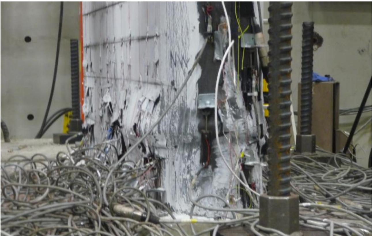
Figure 4: The Local Buckling of the HSS Part at 2.4% Drift
