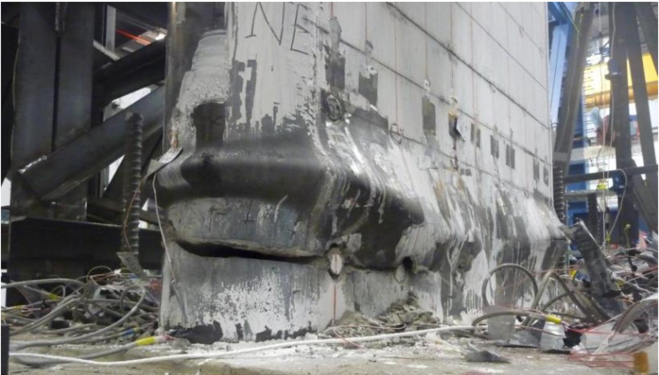
Figure 5: Fracture of the CFSSP-NB1 Specimen East Side at 3.6% Drift
