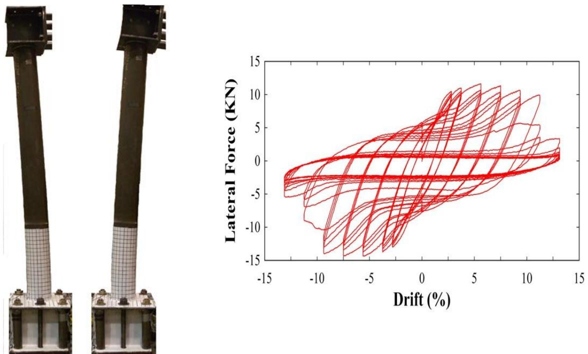
Figure 11: Specimen at Maximum Strength (Left) and Typical Hysteretic Loop (Right)
