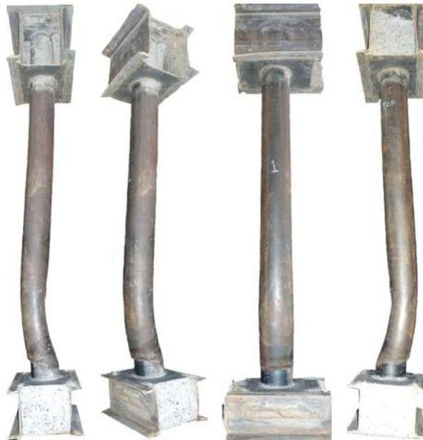
Figure 9. Plastic Deformation of CFDST under Blast
